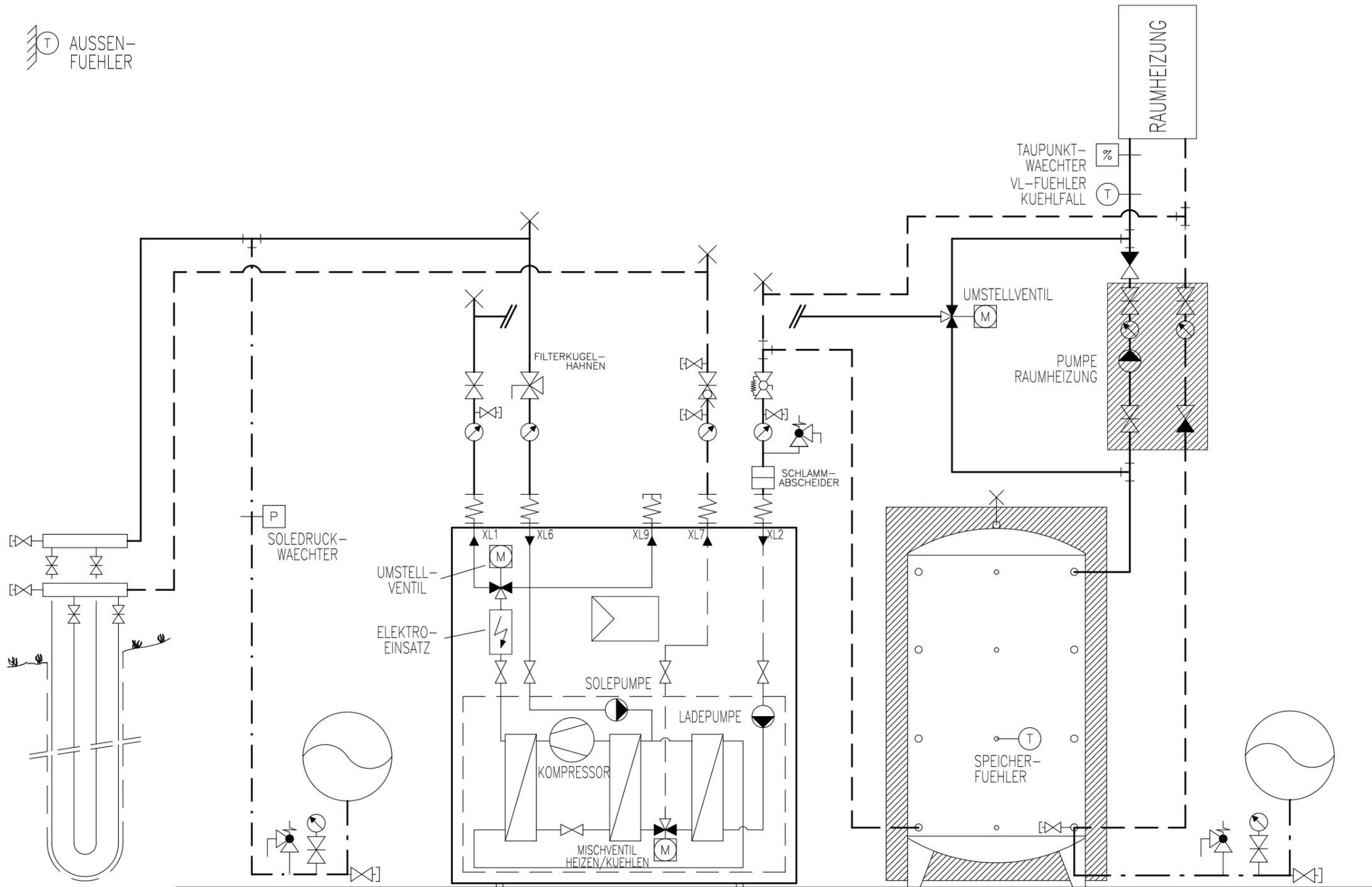
ERDSONDE      EXP.-GEFAESS      WÄRMEPUMPE      SPEICHER      EXP.-GEFAESS
